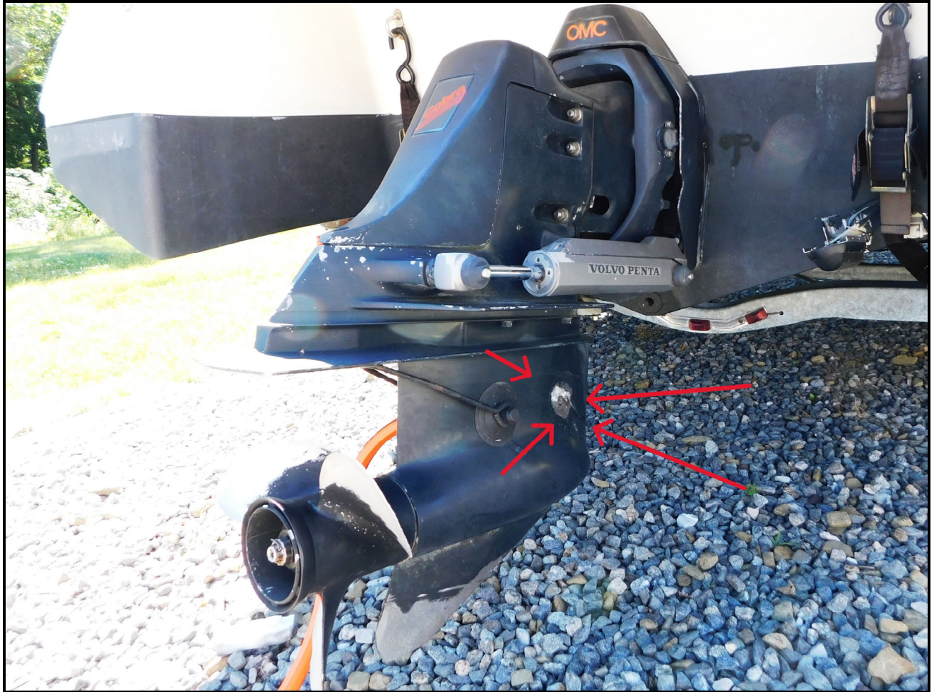
Shows sterndrive unit. Arrows point to observed corrosion spot on lower unit
