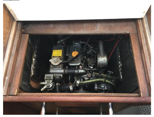
Yanmar 18 hp fresh water-cooled diesel engine
