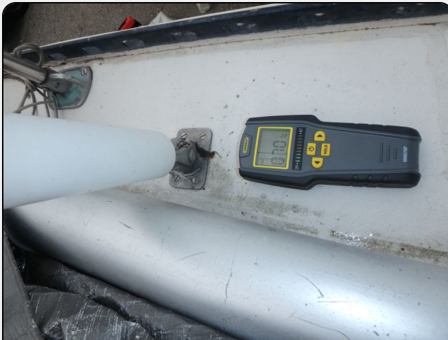
Photo 9: Moisture meter showing a 70% level of moisture around this chainplate penetration on the port side.
