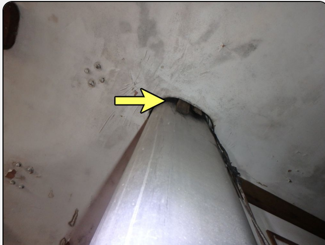
Photo 16: View of the mast where it penetrates the cabin. The wood shims are visible.
