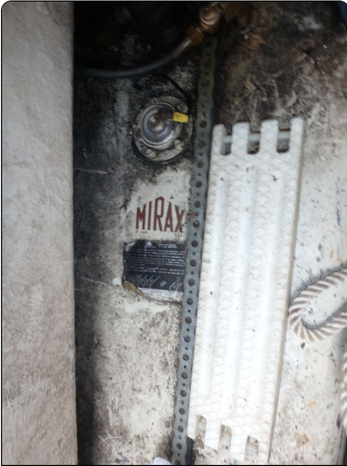
Photo 10 Fuel tank with grounding wire and seacock
