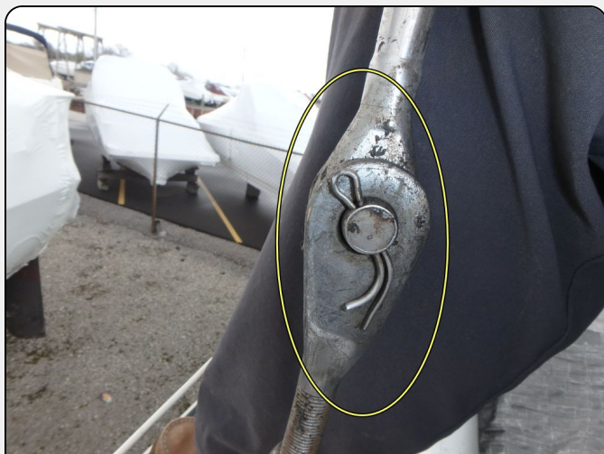
Photo 19: The Stay-Lok eye shows small distress markings on close inspection.
