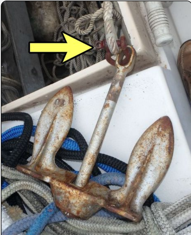
Photo 7: Add thin safety wire through the hole in the anchor pin.
