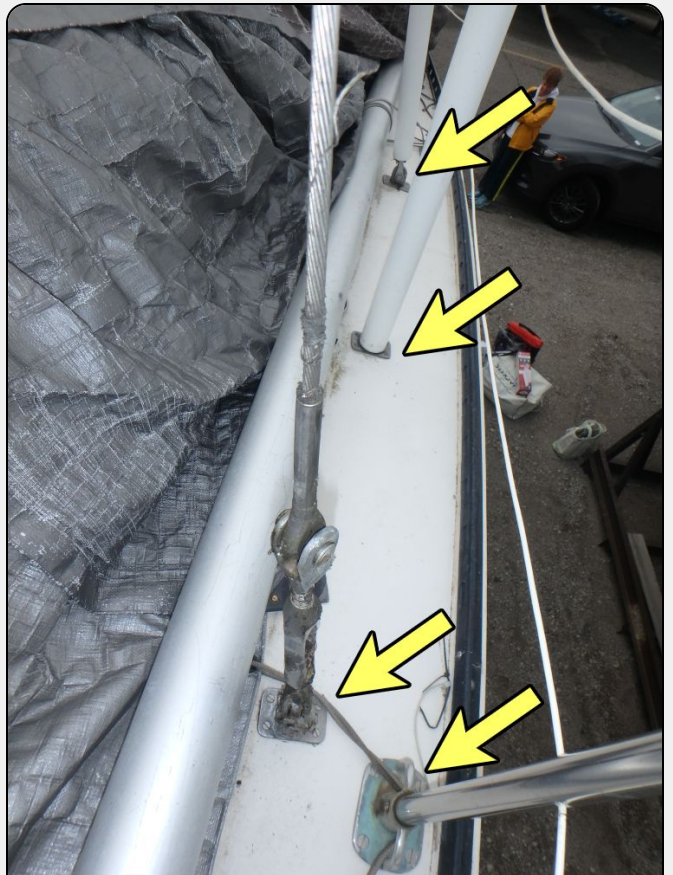
Photo 10: Areas of elevated moisture and delamination were found on the port side decks
