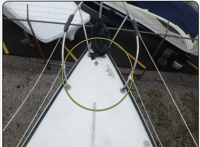
Photo 12: The stanchion bases on the bow should be tightened or rebedded or replaced if necessary
