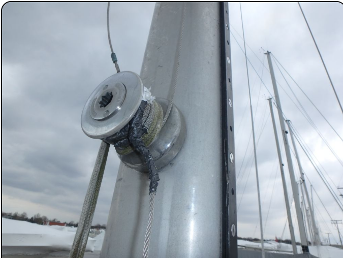
Photo 21: Wire to rope splice for the main halyard.
