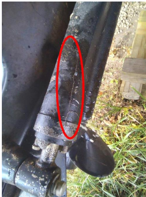
Port Inside Trim Ram Crack
