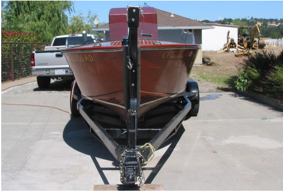
Carvel planked hull; freeboard planking requires service.
