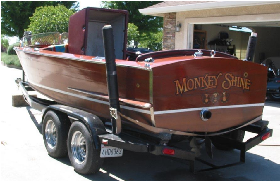
Port quarter carvel freeboard planking overall serviceable.
