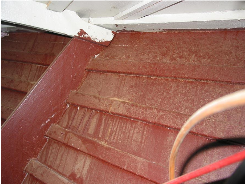
Stbd foredeck clamp shelf hull deck joint secure
