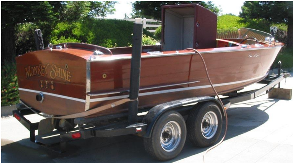
Starboard quarter carvel freeboard planking overall serviceable.
