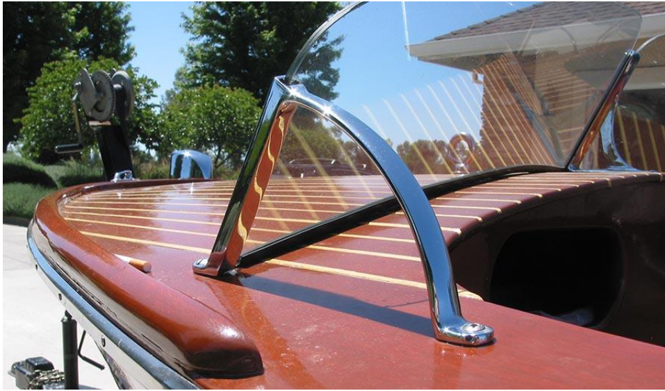
Port foredeck joinery intact & serviceable
