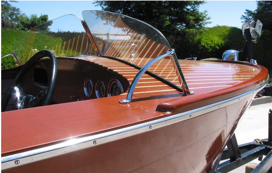
Starboard foredeck joinery intact & serviceable
