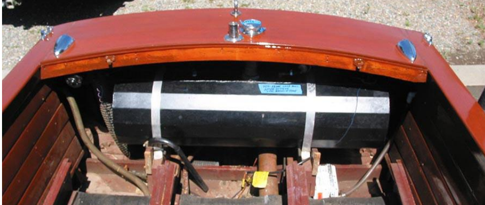
Circa 1954 tern plate steel cylinder fuel tank
