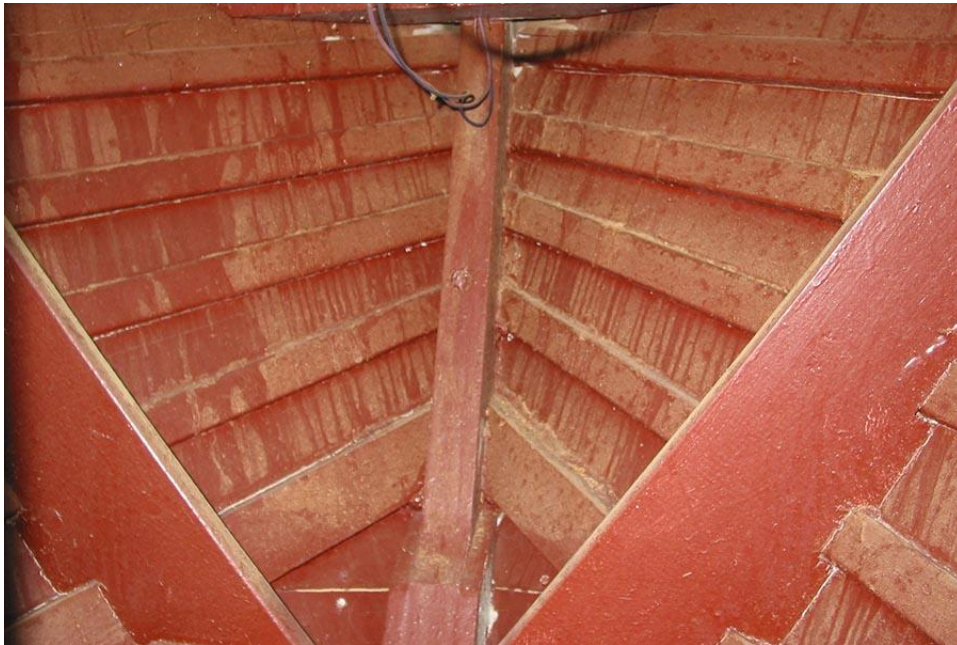
Bow batten & seam construction.
