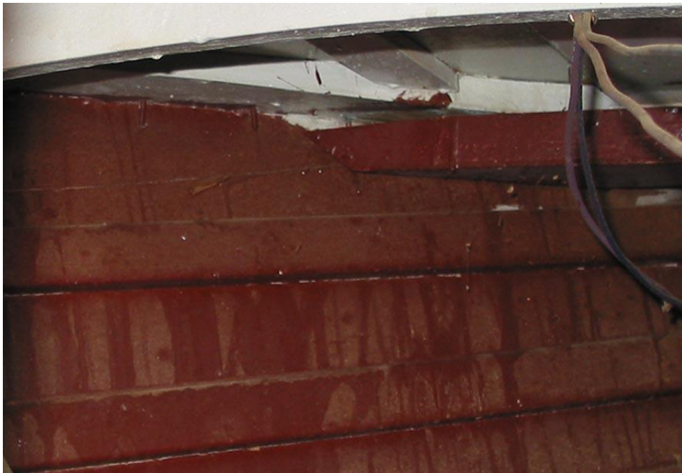
Port foredeck clamp shelf hull deck joint secure
