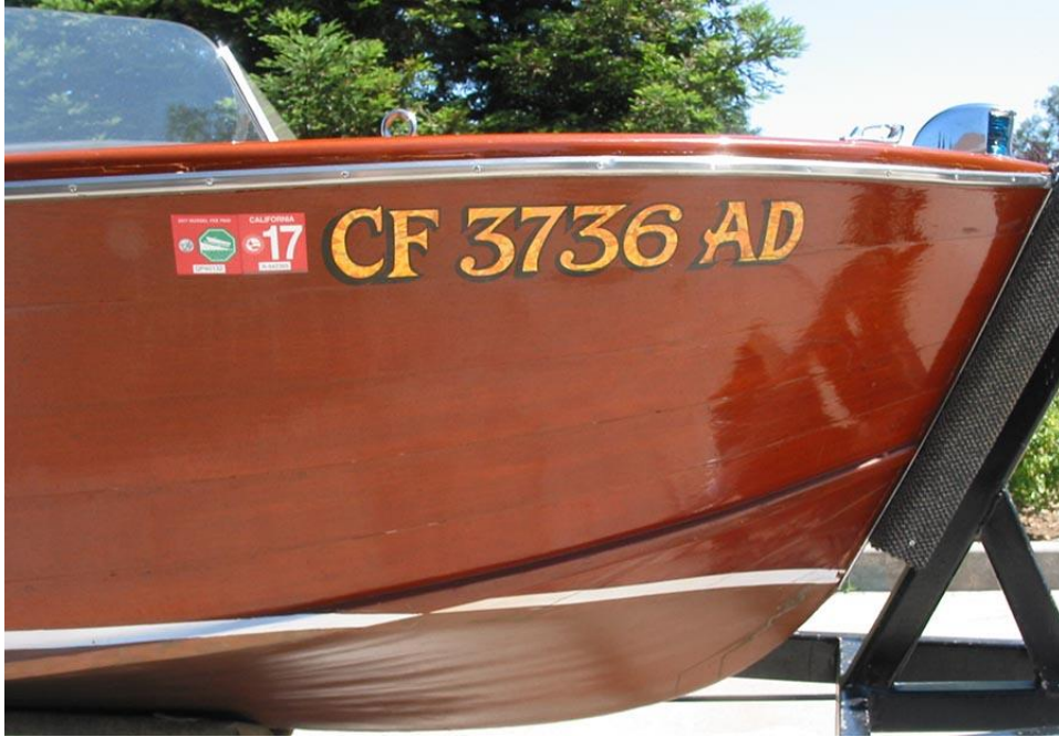
Starboard (stbd) bow freeboard carvel planking, clamp /shelf hull deck joint is intact
