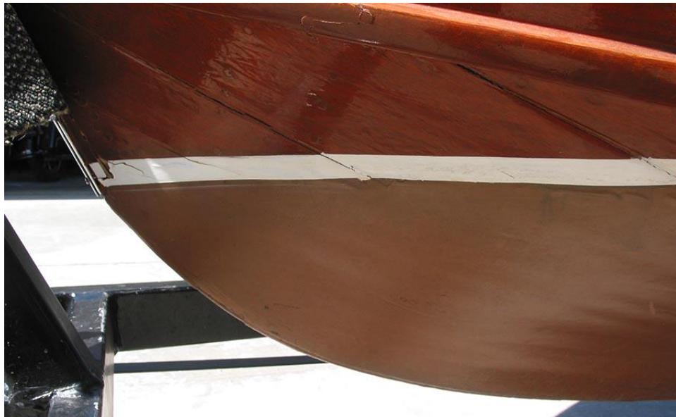
Port bow freeboard carvel planking, clamp/shelf hull deck joint is intact
