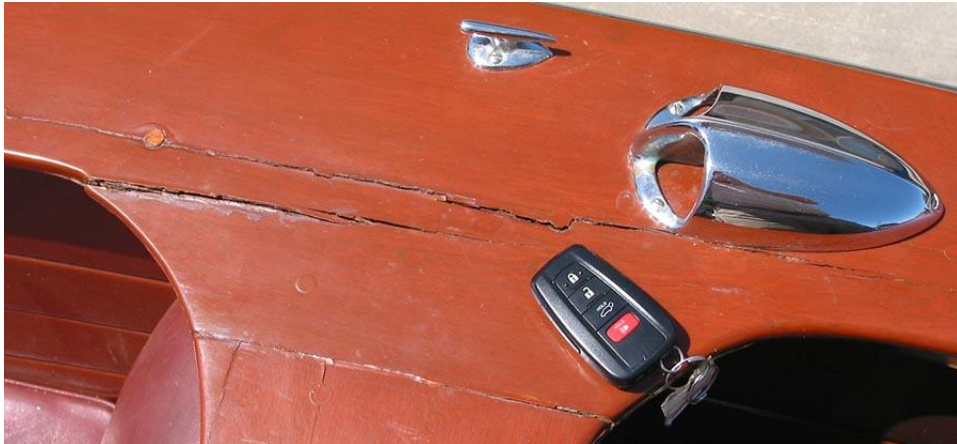
Starboard coverboards are dried, cupping, and cracking.
