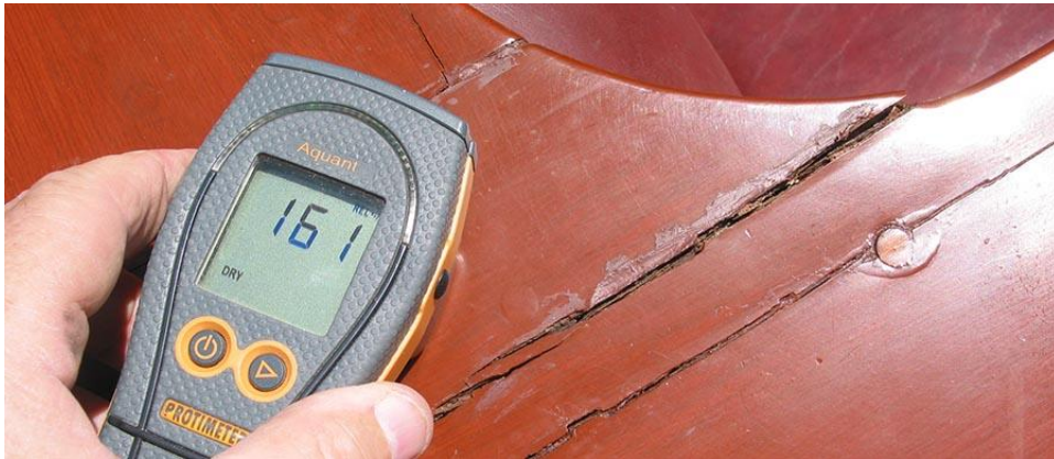
Starboard coverboards are dried, cupping, and cracking.
