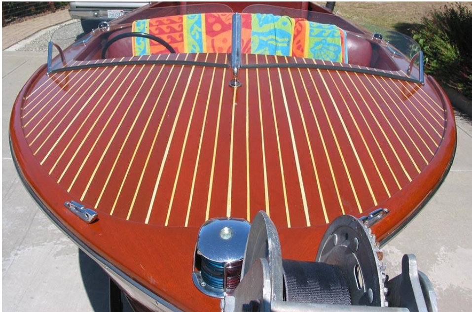
Foredeck payed seam planking & hull carvel planking intact.
