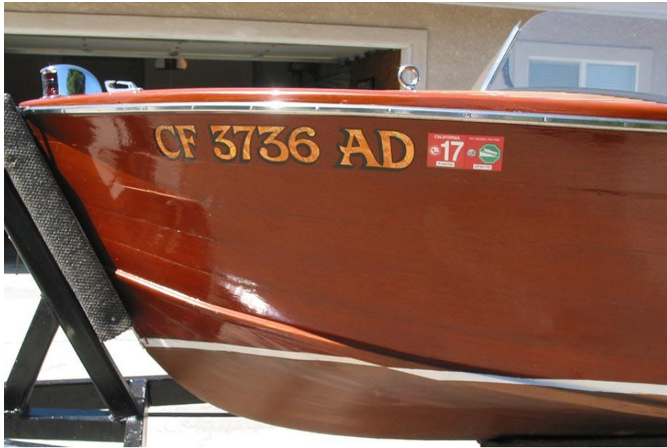
Port bow freeboard carvel planking, clamp/shelf hull deck joint is intact
