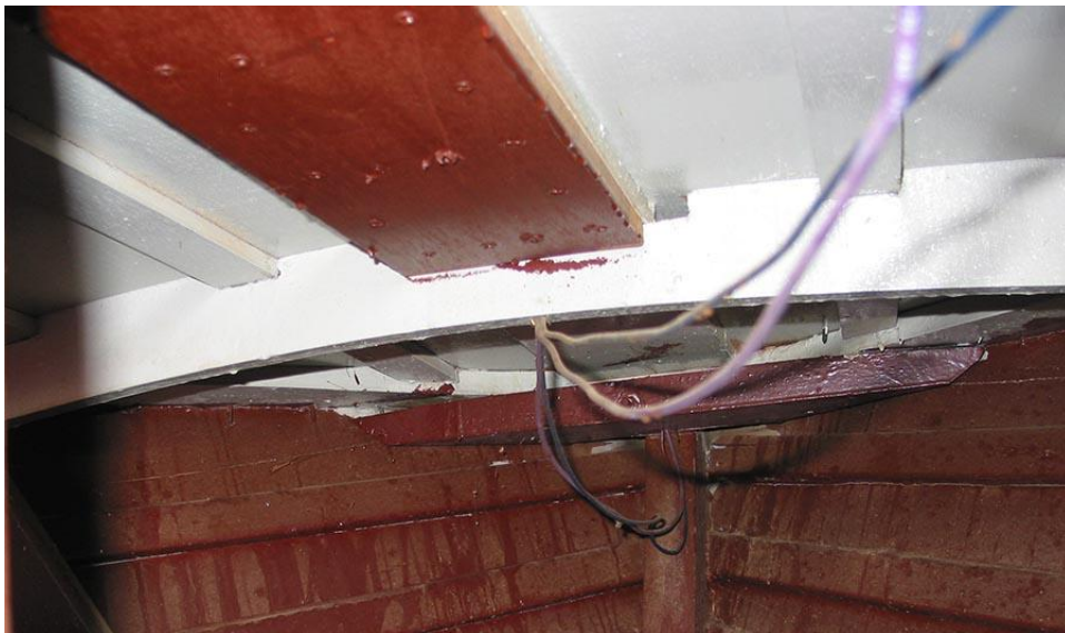
Foredeck transverse deck beams, support battens & plywood sub-deck appear intact.
