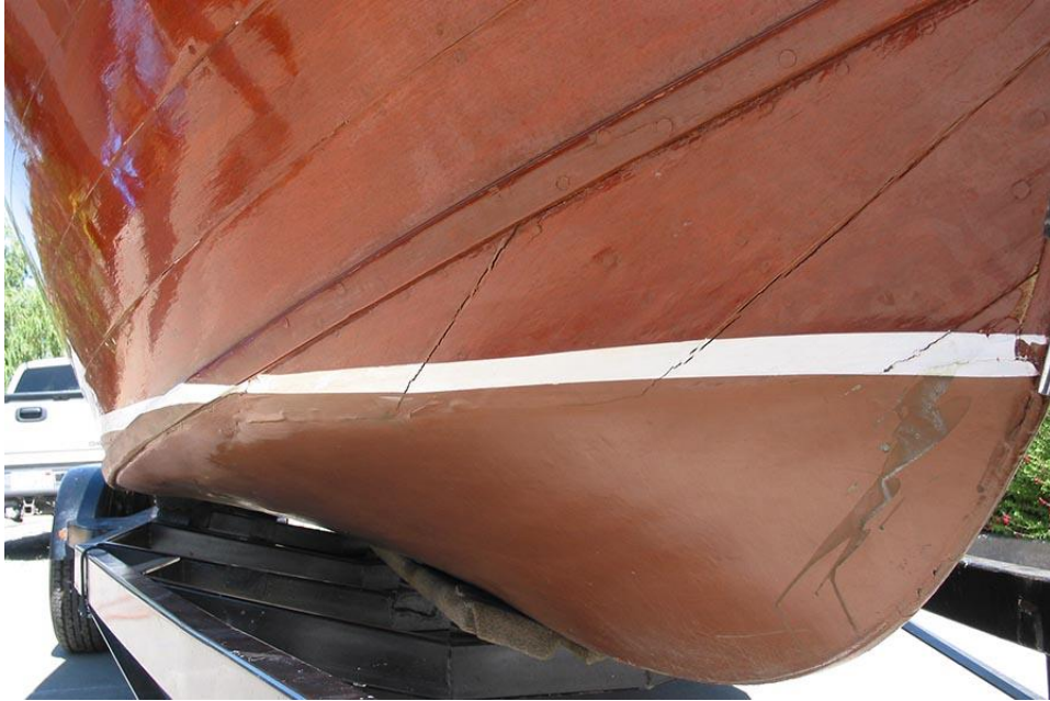
Stbd forefoot scarf joint & plank seams are exposed; the fiberglass overlay is parting from the hull planking.
