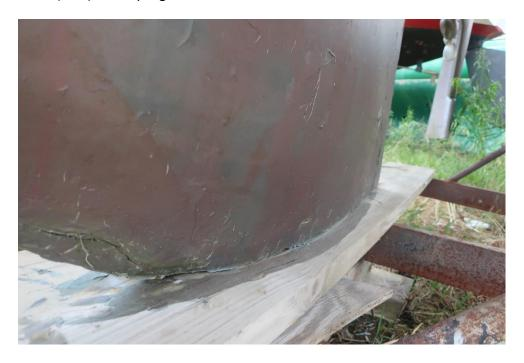
5. Starboard side of keel (percussively dull and delam likely)
