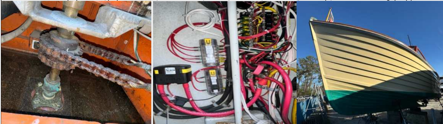
Rudder post, bearings, seals, rudder table, steering cables, chain, conductors and hull are in useful overall condition without wear and tear and well-secured
