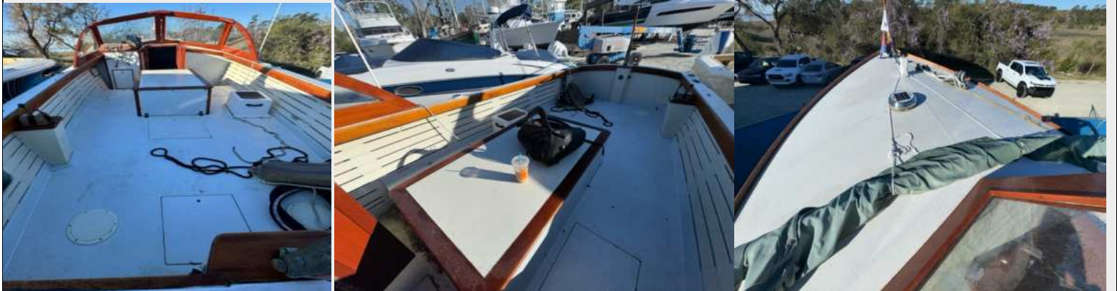
Cockpit, sole, gunwales, coaming, glass windshield panels, engine box, aft control box, foredeck, bimini and cabinhouse are in serviceable condition and structurally sound
