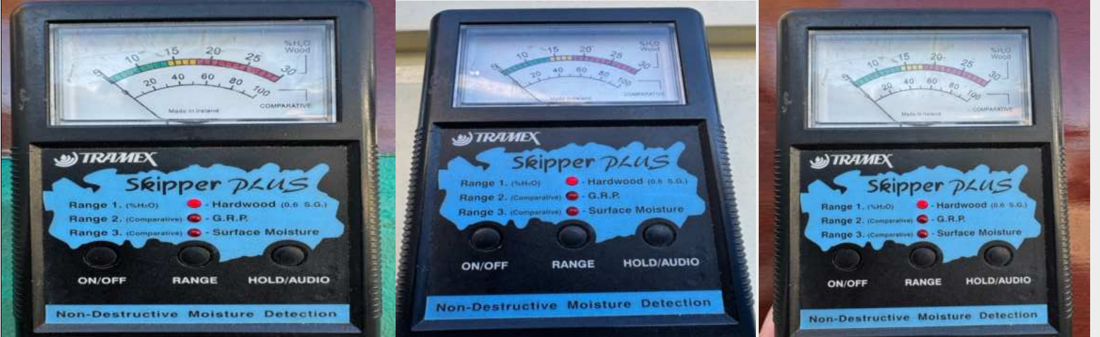
Dry TRAMEX moisture readings were taken on the hull exterior, interior, on deck and structural support members, where accessible
