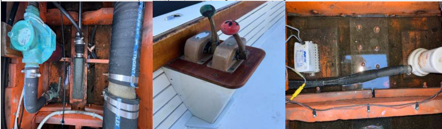
1.25" stainless-steel propeller shaft, propeller shaft seal, bronze thru-hulls, seacocks, sea-strainer, rubber hoses, hoseclamps, aft station and aft bilge pump power on
