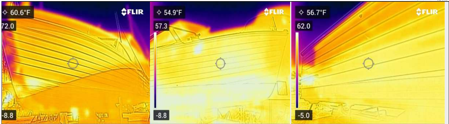
Dry FLIR thermal readings were taken on the hull exterior, interior, on deck and structural support members, where accessible
