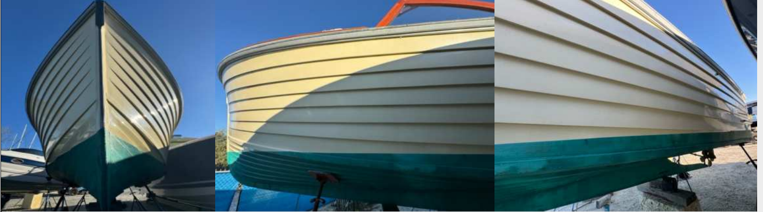
Port and starboard hull exterior, topsides, hulls wetted surface area, keel, stem, planks, fasteners and antifouling bottom paint are in satisfactory structural condition
