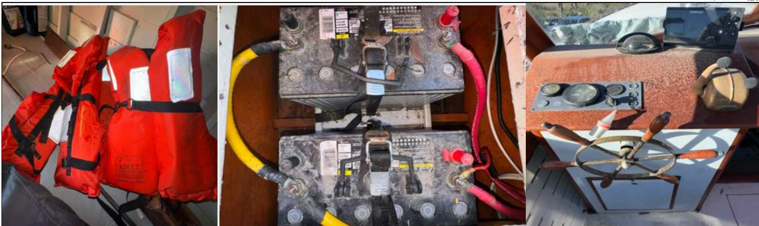
4x US Coast Guard approved type-I adult offshore lifejackets, 2x 12V DC Power-Tec Group 31 AGM batteries and helm station are in serviceable condition
