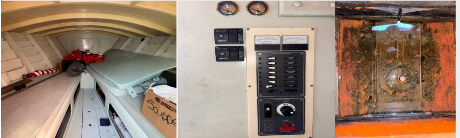
Cuddy cabinhouse interior, cushions, 2x diesel fuel tank level gauges, 2x 12V DC Rule-Mate bilge pump, 12V DC power distribution panel and bilges are in practical shape
