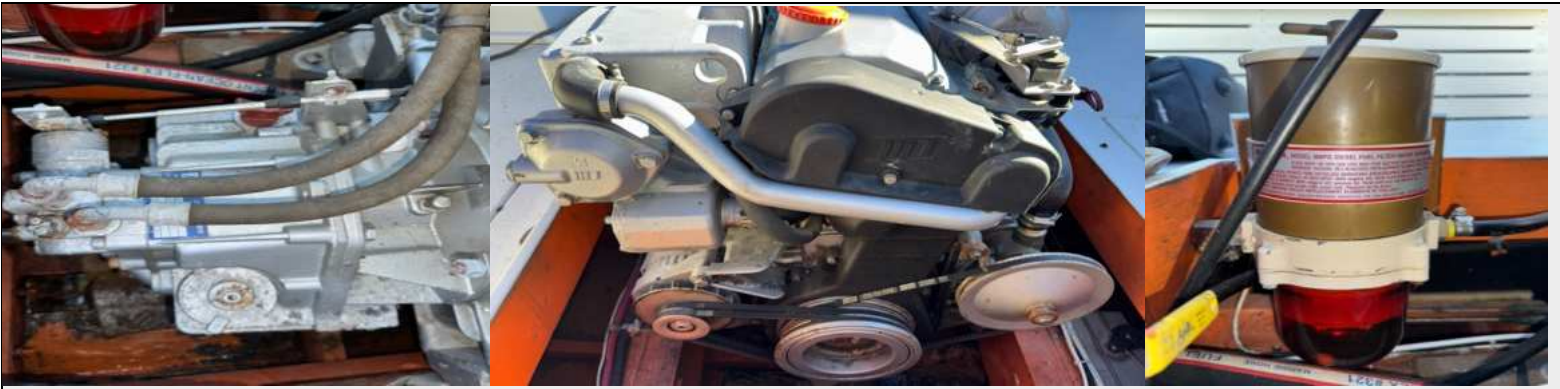
Engine room, Steyr 212HP diesel engine and ZF Hurth marine transmission and Racor diesel fuel-water separating with sightbowl are in serviceable shape
