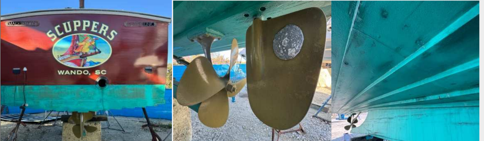
Transom, engine wet-exhaust, sonar transducer, scuppers, 1.25" stainless-steel propeller shaft, strut, cutlass bearing, 4-blade propeller and rudder are in practical shape
