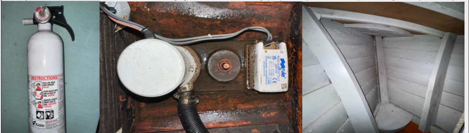
Kidde dry chemical portable fire extinguisher is fully-charged, 2x 12 DC Rule-Mate 2,000 gallon-per-hour bilge pumps and float switches power on chainlocker is secured
