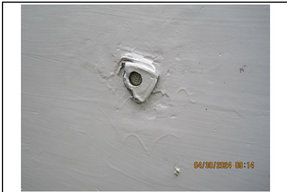
Port hull fuel vent showing some damage.
