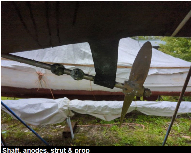
Shaft, anodes, strut & prop
